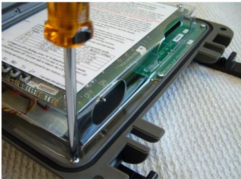
2. With power off, remove the six screws that secure the circuit board holder to the front cover of the camera case.
