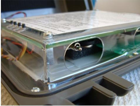
1. The coin battery is located right next to the power switch on the underside of the main circuit board. Be sure the main power switch is **OFF** before replacing the coin battery.
