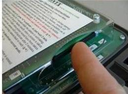
3. Press until CF card seats in holder and edge of card is flush with edge of circuit board.
