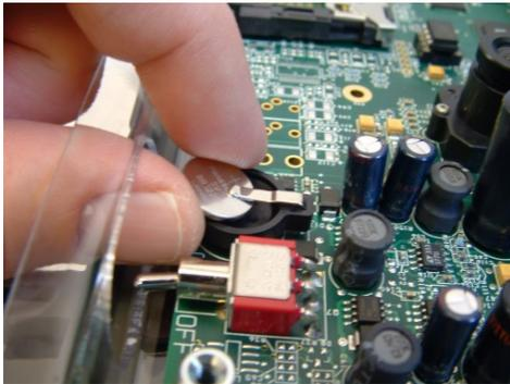
7. Remove battery by grasping between thumb and index finger.
