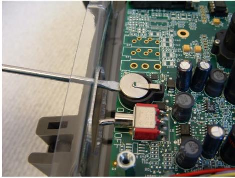
5. Slip a small, flat screwdriver under the coin battery.
