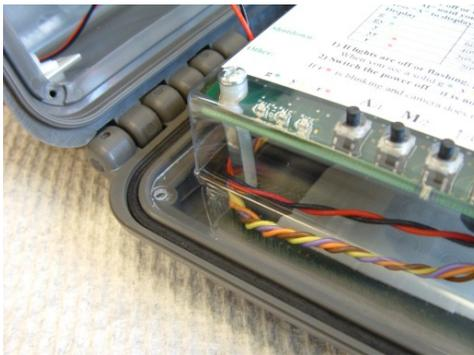
11. Be sure that the wires for power and illuminator route around the outside of the hexagonal standoff in the bottom inside corner of the circuit board holder. Be sure that the holes in the illuminator board match up with the top four holes in the circuit board holder.
