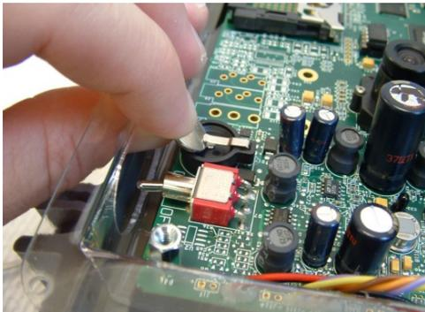
8. Insert a new 3-volt lithium battery (Panasonic BR1225 or equivalent). Be sure that the positive (+) side of the battery faces up. Begin by inserting the battery under the spring clip by tipping the battery at an angle, as shown.
