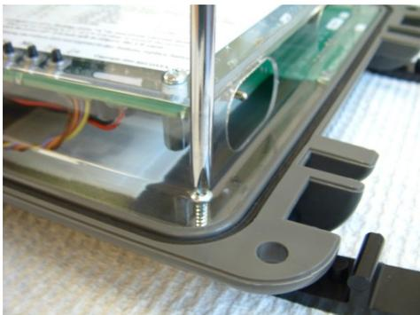
12. Reinstall the six screws that hold the circuit board holder and illuminator in the front cover of the camera case. Tighten screws just until snug; do *not* overtighten or you may strip the threads in the cover.
