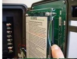
1. Make sure shutdown procedure has been followed and power is off. Then locate the CF card eject button.
