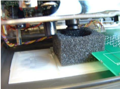
10. Place the circuit board holder in its original position on the front cover of the camera case. Be sure that the lens goes *inside* the lens baffle and that the large capacitor below the lens goes *outside* the lens baffle.
