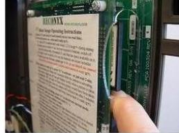
2. Depress eject button until CF card is sticking past edge of circuit board about 1/4 inch.
