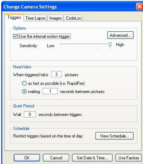
1. Select whether you want to **Use the internal motion trigger** (use the Silent Image internal PIR motion sensor).
