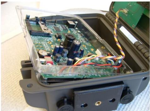
4. You can gently rest the circuit board holder on the main body of the camera case for easy access to the coin battery.
