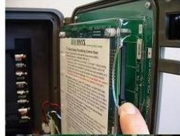
1. Make sure shutdown procedure has been followed and power is off. Then locate the CF card eject button.
