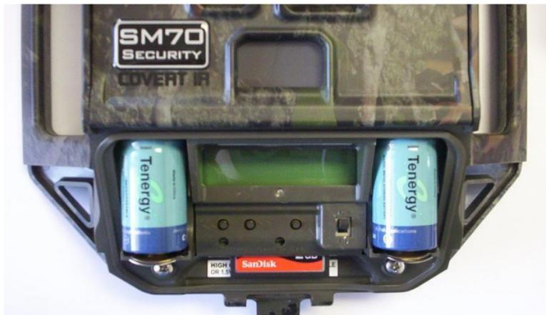
**Warning!** Do not mix battery types! Damage to the camera can result and your warranty will be voided if you mix battery types.
