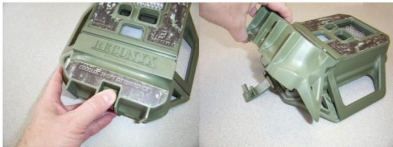
To replace the camera's cover, insert the cover along the bottom edge of the camera's faceplate and rotate it downward until it's flush with the camera. Snap the clasp, pressing firmly in the middle of the clasp, to secure the cover.
