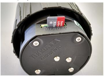
**Warning!** Inserting the memory card upside down or backwards could damage the camera or the memory card. Damage resulting from inserting the card incorrectly is not covered under warranty.
