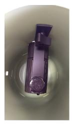
**3.** Mount the camera with bracket inside the cable box using the 3 sided bracket knob.
